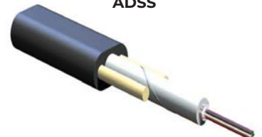
OD: 8.1 x 4.5mm Single-Tube, Gel-Filled Cable 8 F ADSS
